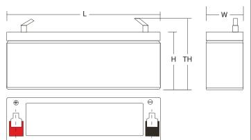
L: 5.28 (134) W: 1.34 (34) H: 2.35 (60) TH: 2.59 (66) Tolerances are +/- 0.04 in. (+/- 1mm) and +/- 0.08 in. (+/- 2mm) for height dimensions. All data subject to change without notice.
