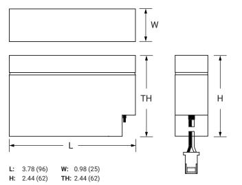
Tolerances are +/- 0.04 in. (+/- 1mm) and +/- 0.08 in. (+/- 2mm) for height dimensions. All data subject to change without notice.
