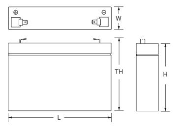
5.91 (150) **W**: 1.34 (34) H: 3.70 (94) TH: 3.94 (100) Tolerances are +/- 0.04 in. (+/- 1mm) and +/- 0.08 in. (+/- 2mm) for height dimensions. All data subject to change without notice.
