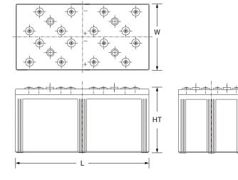
L: 27.90 (709) W: 13.80 (350) H: 13.62 (346) HT: 13.66 (347) Tolerances are +/- 0.04 in. (+/- 1mm) and +/- 0.08 in. (+/- 2mm) for height dimensions. All data subject to change without notice.
