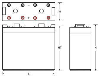
L: 18.70 (475) W: 6.89 (175) H: 13.77 (350) HT: 13.18 (335) Tolerances are +/- 0.04 in. (+/- 1mm) and +/- 0.08 in. (+/- 2mm) for height dimensions. All data subject to change without notice.
