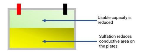
During normal use of the battery the formation of lead sulfate crystals is only temporary, they disperse during the recharging process. The issue with sulfation occurs when the larger lead sulfate crystals become permanent.
