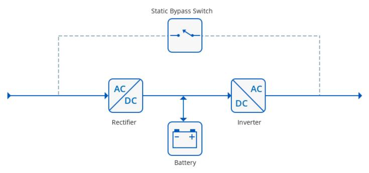
Specializing in online UPS Power Sonic provides a number of online double conversion UPS systems including rack-mount options, from 1kVA to 1000kVA with a vast array of applications and features. Ranges include the PowerPower RT, PowerClever and PowerLevel..
