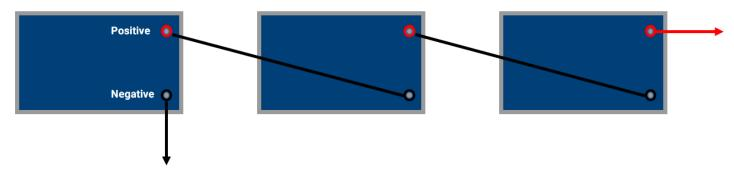
Sealed lead acid batteries have been the battery of choice for long string, high voltage battery systems for many years, although lithium batteries can be configured in series it requires attention to the BMS or PCM.
