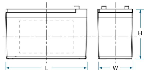
**Dimensional Tolerances** +/- 0.04 in. (+/- 1mm) for length and width
