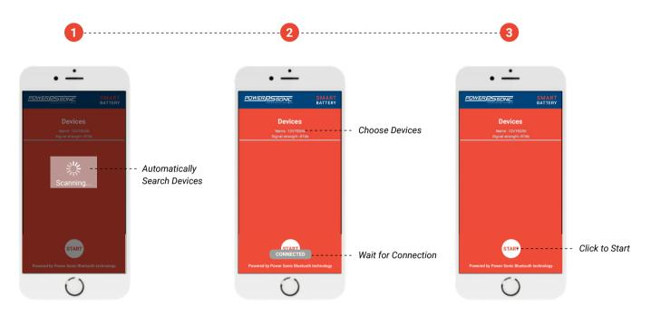
If you have selected a battery to connect with and the app is not confirming the connection, it may be because someone else has already connected to the battery. Only one device can be connected to a battery at any one time.
