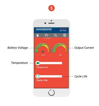
"Engineers Special" when inputting the password as 1234 you can see each series voltage. When inputting 5678 you can rename the connected battery.
