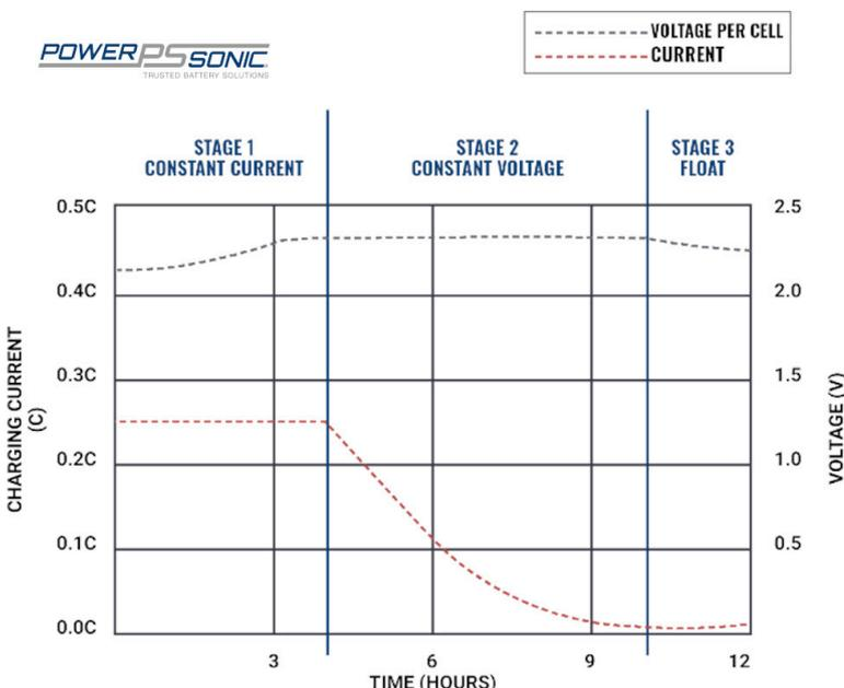
Stage 1, as shown above, the current is limited to avoid damage to the battery. The rate of change in voltage continually changes during Stage 1 eventually beginning to plateau when the full charge voltage limit is approached. The constant current/Stage 1 portion of the charge is crucial before moving onto the next stage. Stage 1 charging is typically done at 10%-30% (0.1C to 0.3C) current of the capacity rating of the battery or less.
