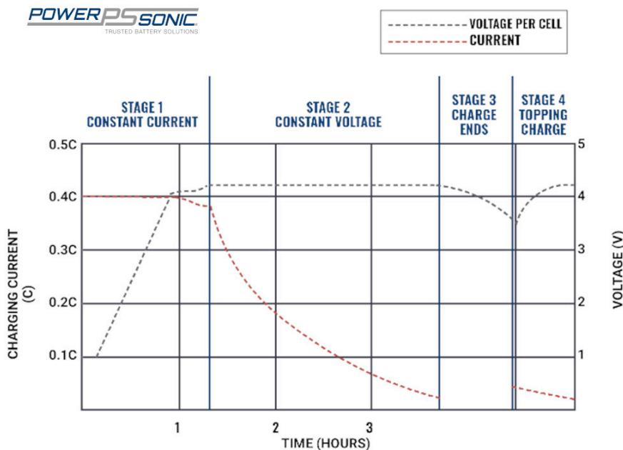
Stage 1 battery charging is typically done at 30%-100% (0.3C to 1.0C) current of the capacity rating of the battery. Stage 1 of the SLA chart above takes four hours to complete. The Stage 1 of a lithium battery can take as little as one hour to complete, making a lithium battery available for use four times faster than SLA.
