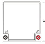
6.55 (166.5) W: 6.88 (175) H: 4.64 (118) HT: 4.92 (125) Tolerances are +/- 0.04 in. (+/- 1mm) and +/- 0.08 in. (+/- 2mm) for height dimensions. All data subject to change without notice.
