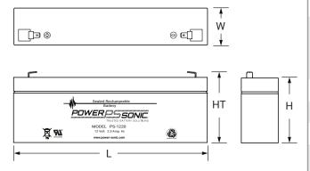
L: 7.00 (178) W: 1.37 (35) H: 2.36 (60) HT: 2.59 (66) Tolerances are +/- 0.04 in. (+/- 1mm) and +/- 0.08 in. (+/- 2mm) for height dimensions. All data subject to change without notice.
