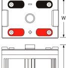
L: 6.88 (175) W: 8.26 (210) H: 12.99 (330) HT: 13.77 (350) Tolerances are +/- 0.04 in. (+/- 1mm) and +/- 0.08 in. (+/- 2mm) for height dimensions. All data subject to change without notice.
