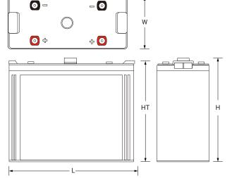
**L**: 18.70 (475) **W**: 6.89 (175) **HT:** 13.26 (337) **H:** 13.77 (350) Tolerances are +/- 0.04 in. (+/- 1mm) and +/- 0.08 in. (+/- 2mm) for height dimensions. All data subject to change without notice.
