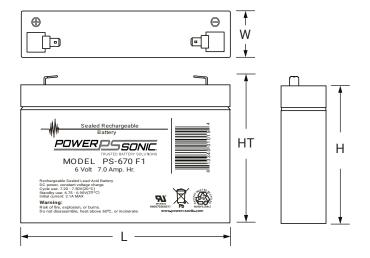
L: 5.95 (151) W: 1.34 (34) H: 3.70 (94) HT: 3.94 (100) Tolerances are +/- 0.04 in. (+/- 1mm) and +/- 0.08 in. (+/- 2mm) for height dimensions. All data subject to change without notice.
