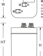
2.64 (67) W: 2.64 (67) H: 3.94 (100) HT: 4.64 (118) Tolerances are +/- 0.04 in. (+/- 1mm) and +/- 0.08 in. (+/- 2mm) for height dimensions. All data subject to change without notice
