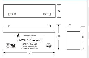
**L**: 5.28 (134) **W**: 1.34 (34) **H**: 2.35 (60) HT: 2.56 (65) Tolerances are +/- 0.04 in. (+/- 1mm) and +/- 0.08 in. (+/- 2mm) for height dimensions. All data subject to change without notice.
