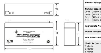
**L**: 7.00 (178) **W**: 1.38 (35) **H:** 2.36 (60) Tolerances are +/- 0.04 in. (+/- 1mm) and +/- 0.08 in. (+/- 2mm) for height dimensions. All data subject to change without notice.
