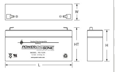
7.00 (178) **W**: 1.38 (35) **H**: 2.36 (60) **HT**: 2.60 (66) Tolerances are +/- 0.04 in. (+/- 1mm) and +/- 0.08 in. (+/- 2mm) for height dimensions.
