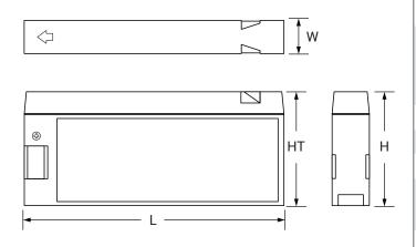
L: 7.17 (182) W: 0.94 (24) H: 2.40 (61) HT: 2.40 (61) Tolerances are +/- 0.04 in. (+/- 1mm) and +/- 0.08 in. (+/- 2mm) for height dimensions. All data subject to change without notice.
