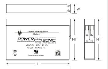
**L**: 5.91 (150) **W**: 0.80 (20) **H**: 3.52 (89) HT: 3.52 (89) Tolerances are +/- 0.04 in. (+/- 1mm) and +/- 0.08 in. (+/- 2mm) for height dimensions. All data subject to change without notice.
