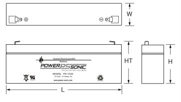
L: 5.28 (134) W: 1.34 (34) H: 2.35 (60) HT: 2.56 (65) Tolerances are +/- 0.04 in. (+/- 1mm) and +/- 0.08 in. (+/- 2mm) for height dimensions.
