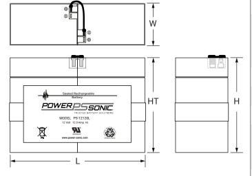
**L**: 8.45 (215) **W**: 2.75 (70) **H:** 5.75 (146) **HT**: 5.75 (146) Tolerances are +/- 0.04 in. (+/- 1mm) and +/- 0.08 in. (+/- 2mm) for height dimensions.
