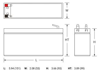
Tolerances are +/- 0.04 in. (+/- 1mm) and +/- 0.08 in. (+/- 2mm) for height dimensions. All data subject to change without notice.
